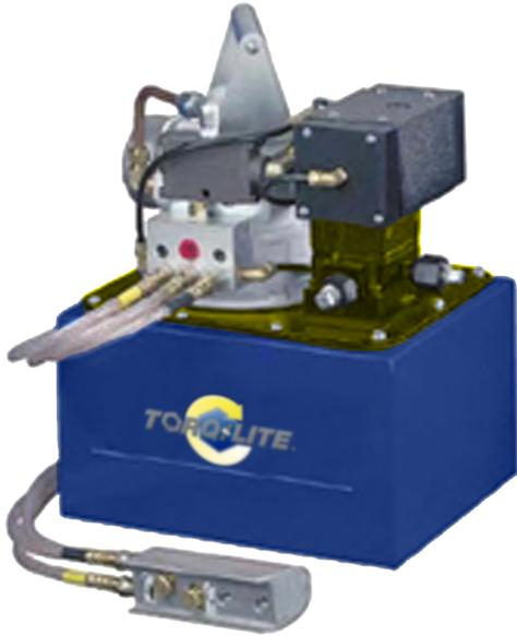
The JNAHC-AHR series pump is a rotary-style air motor and should be used where air is the preferred source of energy. It has a 3hp motor when it is starting under full load and two-speed operation for rapid cylinder advance. This pump features a remote with full control over advance and return. The tandem center holds the load when the pump is shut off.
