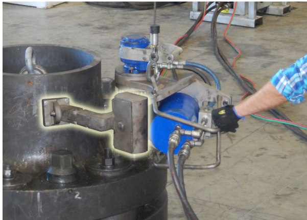
Inline Reaction Member Reacts off of the riser
