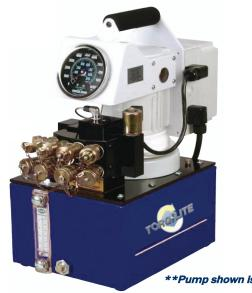
The JNEHC-10 is a heavy duty electric pump made for multiple applications with a low voltage starting potential. The pump features a 10' remote motor control with full control over advance, hold and retract operations. The tandem center holds the load when the pump is shut off. True unloading valve achieves greater pump efficiency, allowing higher flow at maximum pressure.
