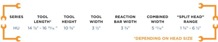
The HU Tool will work on any standard torque wrench pump, eliminating the need to purchase a special unit to operate it.
