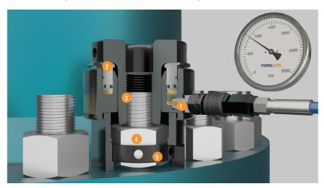
1 Hydraulic oil flows into load cell
