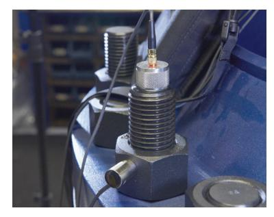
Measurement is achieved by determining the change in the transit time of an ultrasonic shock wave along the length of the fastener as it is tightened.
