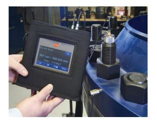
The Echometer Premier ultrasonic measurement device has been developed specifically for the bolting industry which measures, displays, stores and transfers bolt elongation and load. A hard wearing unit with a touch screen. The most advanced instrument available to control or verify bolt elongation and load in the field or laboratory developed with input from the most experienced users and electronic developers in the bolt tightening industry delivering a system with intuitive software.
