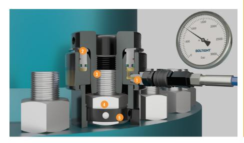
Hydraulic oil flows into load cell
