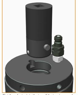
Slot the adaptor into the top of the tensioner and rapidly wind down onto the stud using a square drive wrench or impact gun.
