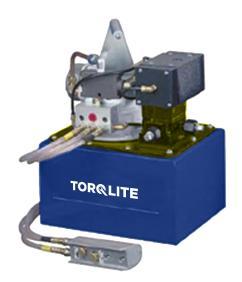
The JNAHC-AHR series pump is a rotary style air motor and should be used where air is the preferred source of energy. It has a 3hp motor when it is starting under full load and two-speed operation for rapid cylinder advance. This pump features a remote with full control over advance and return. The tandem center holds the load when the pump is shut off.
